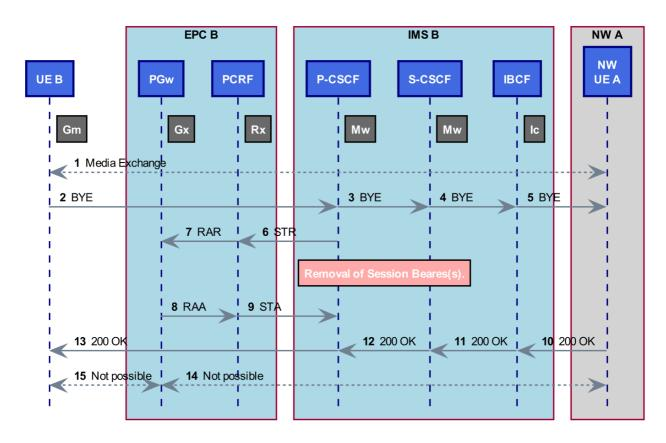
NOTE: The Rx exchange need not wait for the Gx exchange to complete.
