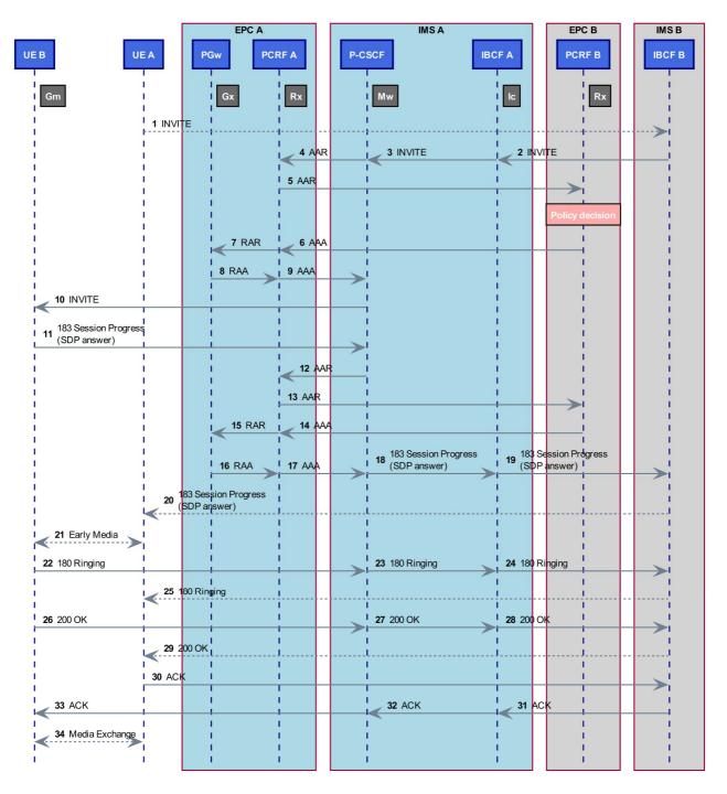
NOTE 1: Call is routed towards NWK B and originating roaming TD\_VxLTE\_RMI\_INI\_01 or originating interoperability TD\_VxLTE\_INT\_INI\_01 scenario may be checked for NWK UE A.
