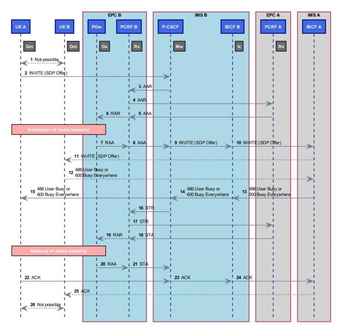
NOTE: Dashed connections between UE B and IBCF A represent the signalling which passes different entities but due to the scope of TD those are not points of observation.
