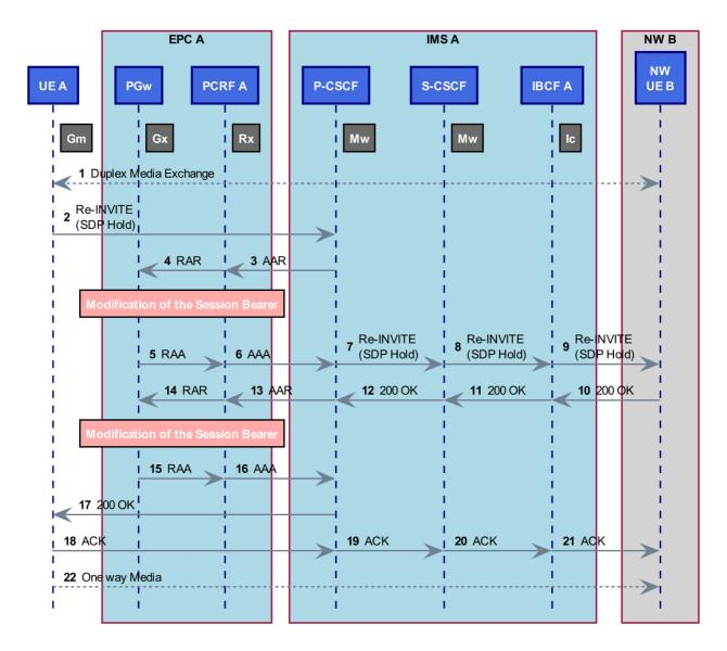
NOTE 1: A SIP UPDATE message may also be used instead of re-INVITE to initiate a new offer/answer exchange. NOTE 2: The Rx exchange need not wait for the Gx exchange to complete.
