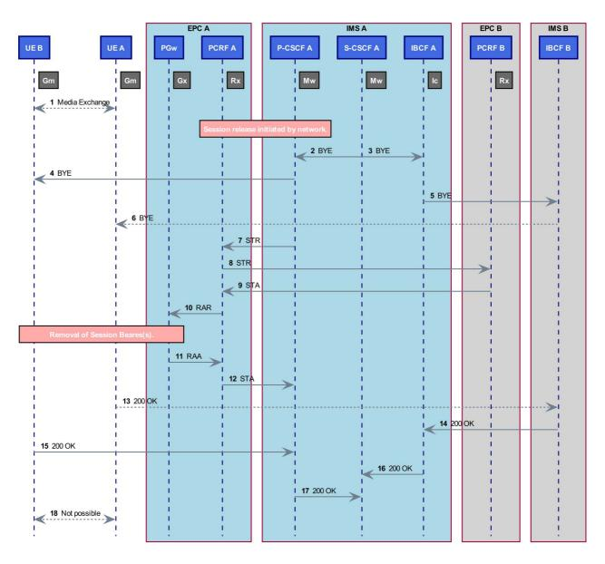
NOTE 1: The Rx exchange need not wait for the Gx exchange to complete.
